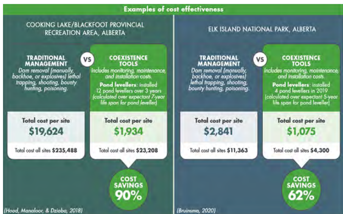
Figure 32: Example calculations of cost savings of flow devices at two locations in Alberta, Canada, from the Miistakis Institute Fact Sheet: Cost-benefit Analysis of Beaver Coexistence Tools .
